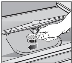
Return the combination filter so that it lies flat in the base of the dishwasher. Secure it by turning the handle clockwise.
